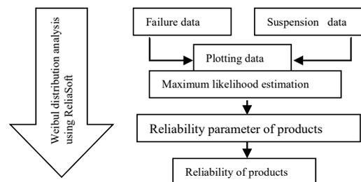
**Figure 1.** Reliability analysis steps of the remanufactured computer
