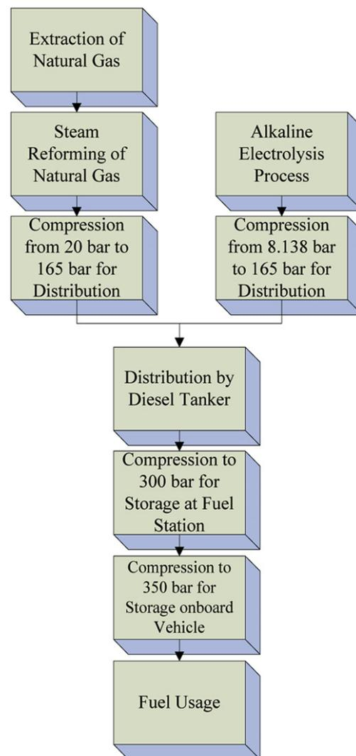
Fig. 1 – Simplified block diagram for hydrogen fuel life cycle models.
